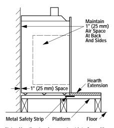
Note: Hearth extensions must not interfere with circulating grillwork
